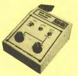
Using any source of composite video (colour or monochrome) and the Watford Beeb Video Digitiser, you can convert an image from your camera into a graphics screen on the BBC Micro.
