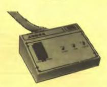
Adder is the ultimate EPROM programmer for the BBC Micro. It will program many different EPROMs up to the very latest 27256 32K devices.
