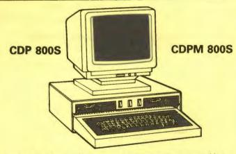
Twin 800K Double sided 40-80 track switchable disc drives mounted in an attractively finished Beige colour plinth for the BBC Micro. Supplied complete with integral power supply, cables and Utilities disc. The switches are mounted on the front panel for ease of use.
