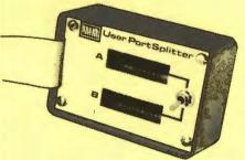
Gone are the days when you had to plug and unplug devices from the User Port. This extremely useful little device allows two units to be connected to the User Port simultaniously, and select between them simply by toggling a switch. This device is particularly useful for those people using Quest Mouse and the Watford Video Digitiser or any similar combination. Excellent Value at £15
